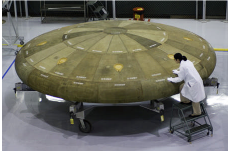
This is the Thermal Protection System Manufacturing Demonstration Unit developed for NASA's Orion Crew Exploration Vehicle project.
